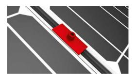
Fix the module in place at the end of a row with universal module end clamp OneEnd. Klick the Stance in the notches. Alternatively use the standard end clamp. Insert the MK2 nut into the mounting rail and turn clockwise by 90°. Place clamps on the module frames and fix them. Never mount module end clamps directly on the rail joint or end of the rail! (Spacing: min. 50 mm from edge of module frame). Pay attention to the mounting instructions by module manufacturer!
