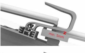
Flex deck tiles and lower tiles in the area of the hanger. The top edges of a horizontal row must be at the same height.
