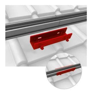
Lay Mounting Rail on joint with rail connector and connect with T bolts and self-locking nuts. The rail joint may not be in the range of the roof fastener.
