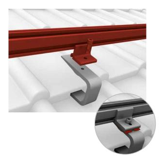
The Mounting Rail is mounted on to the roof fastener using K2 Climbers and K2 Bolts with serrated under head. Tightening torque 16 Nm.
